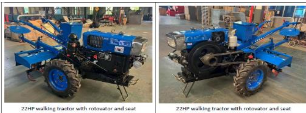
Figure 10a and 10b 22 hp hand walking tractor with rotovator and seat specs in the figure below
