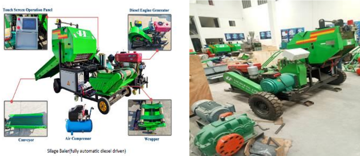
Figure 6 a & 6b Silage baler with conveyor. Left figure details of the baler. Right the silage baler at the warehouse in Nairobi.
