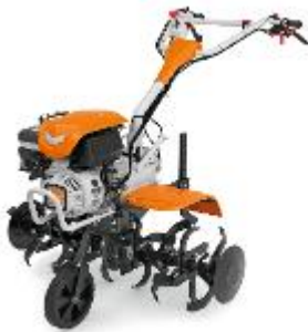
Figure 8. A light hand walking tractor that can be used for land cultivation and weeding in between the rows.
