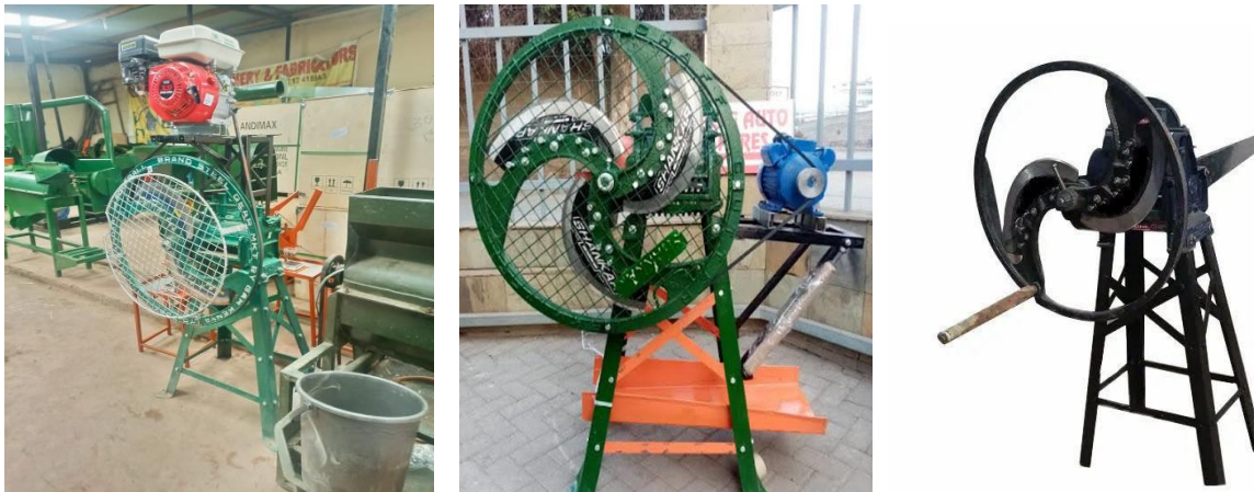
Figure 5a, 5b & 5c showing petrol, electric and manual powered chaff cutters. These are very strong and hardy farm implements which can easily be maintained and repaired by farmers themselves or a local technician.
