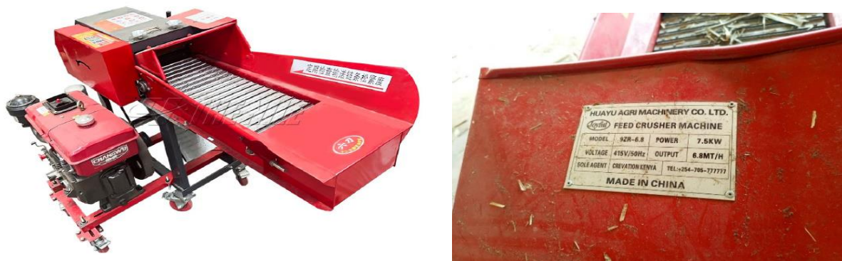
Figure 4 a & 4b Forage chopper with conveyor. Right figure detail with specs
