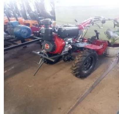
Figure 9. A heavier hand walking tractor that can be used for land cultivation.
