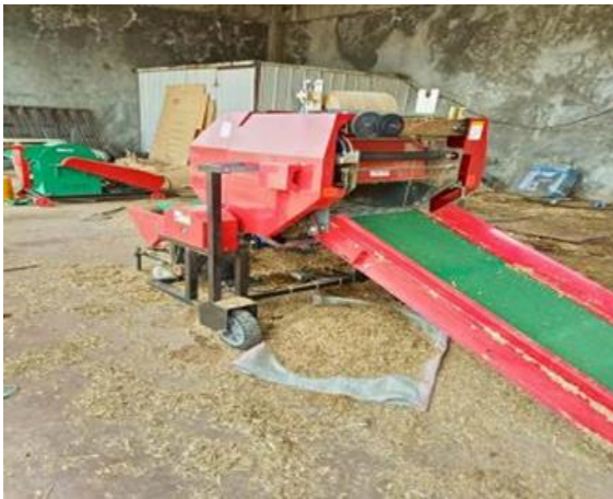
Figure 7. Silage baler with conveyor at Crevation International on the right the baler in the field
